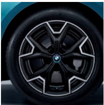
18inch aluminum alloy wheels Yspoke881type, two-color
